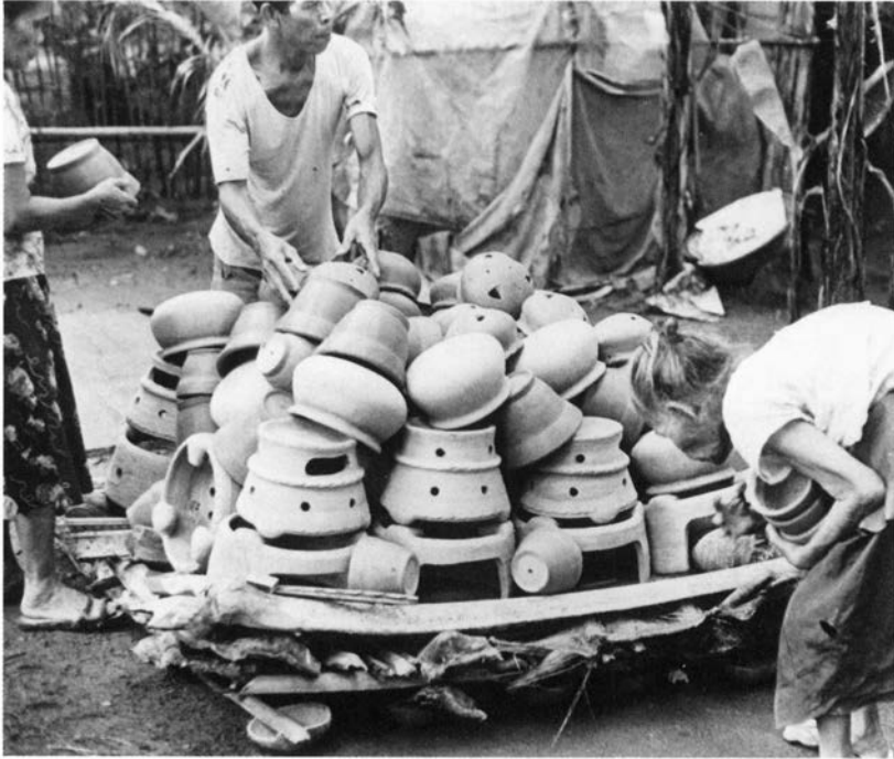
FIGURE 9.3. Pots made by three women are stacked for firing on a frame of coconut fronds, bamboo poles, and coconut husks. The stoves are placed on the bottom, then cooking pots and flowerpots; all are inverted.
